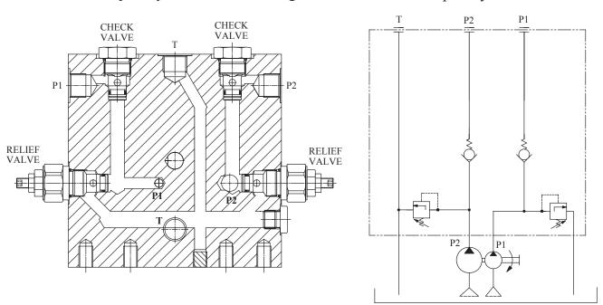
The W85BT series power pack is designed for applications that need two independent hydraulic power supply, but only use a single transmission.
